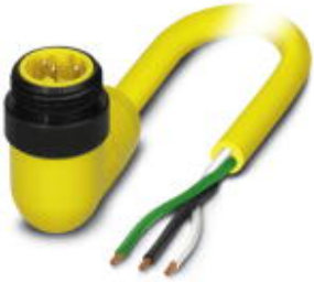
Power cable, 3-position, PVC, yellow, Plug angled 7/8"-16UNF, A - standard, on free cable end, A - standard, cable length: 5 m
