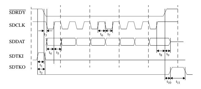
Figure 6. SD Port Read Timing
