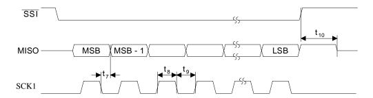
Figure 5. MISO Read Timing in SPI Slave Mode
