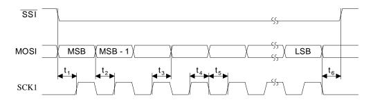
Figure 4. MOSI Write Timing in SPI Slave Mode
