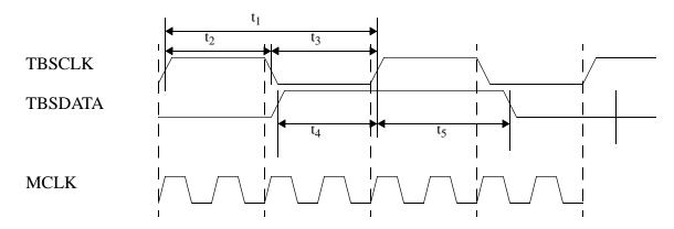
Note: Example timing shown for a 256 kHz output rate and no programmable delays.
