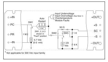
*Figure 3* — *PC/SC module alarm logic.*
