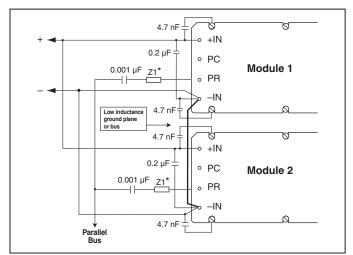
*Figure 9* — *AC coupled single-wire interface.*
