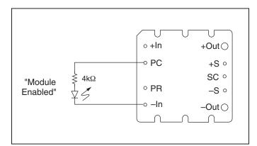
Figure 4 — LED on-state indicator.
