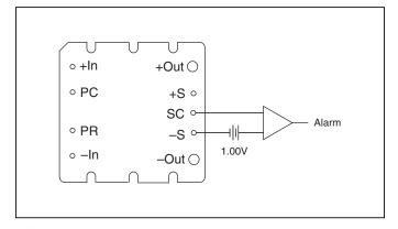
*Figure 7* — *Secondary side on-state indicator.*
