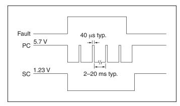
*Figure 5* — *PC/SC module alarm timing.*
