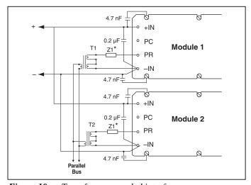
Figure 10 — Transformer-coupled interface.
