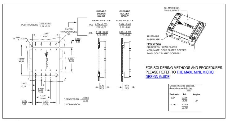
Figure 13 — PCB mounting specifications
