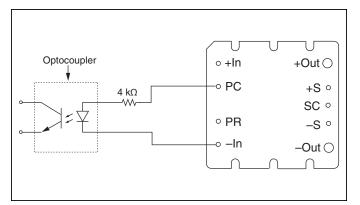
Figure 6 — Isolated on-state indicator.
